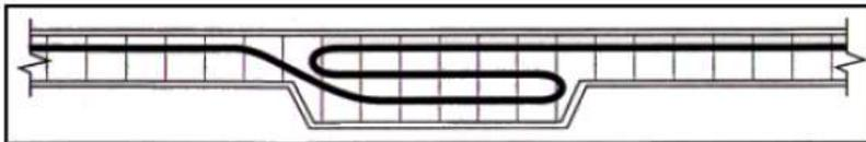
*Fig. 3 Installation practice to provide surplus cable length (cable slack) for small diameter cables in a cable tray run. Installation shows ladder type cable trays with reducers between the different widths of cable tray. Bending radii of the cable must not violate the cable manufacturer's recommendations.*
