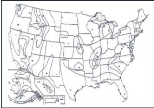
*Fig. 1 The 0 to 4 values show the relative earthquake potential magnitude areas. These values are related to the seismic zone factors that are used for earthquake design requirements. For additional information see the "Uniform Building Code."*
